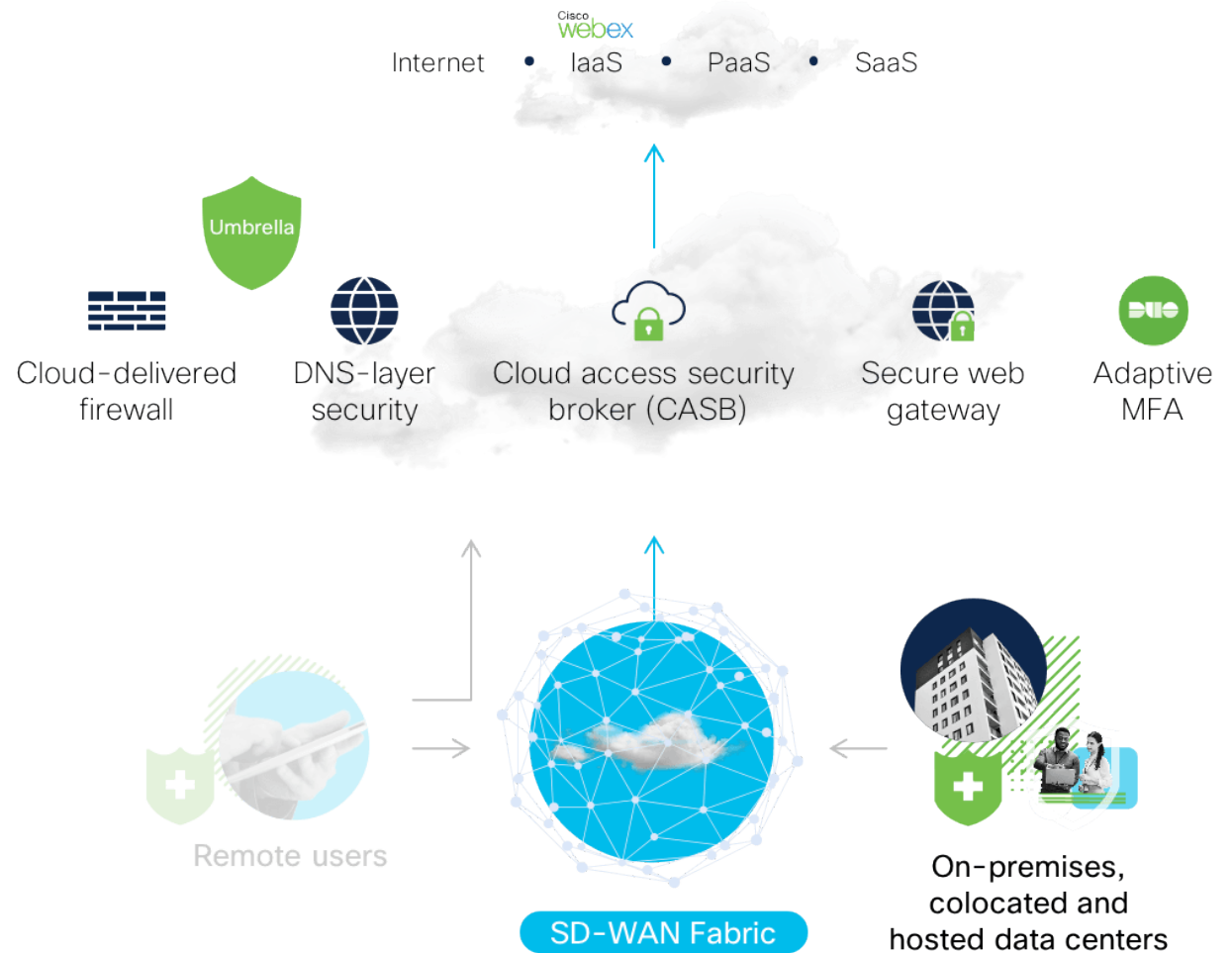
Figure 3: Cisco SD-WAN enabled branch architecture.
