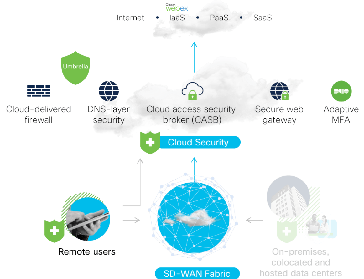
Figure 2: Cisco secure remote access architecture.
